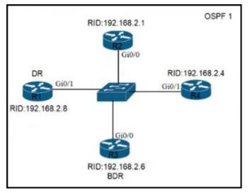
Refer to the exhibit. All routers in the network are configured R2 must be the DR. After the engineer connected the devices, R1 was elected as the DR.
