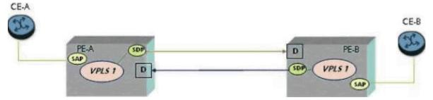
Assume the port on CE-A is sending two tags, a top tag of 100 and a bottom tag of 500. PE-A is configured with a SAP id of 1/1/1:100.\*.
