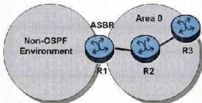
In the topology shown, router R1 is an ASBR configured to export external routes to OSPF. How many type 4 LSAs will be present in the network?
