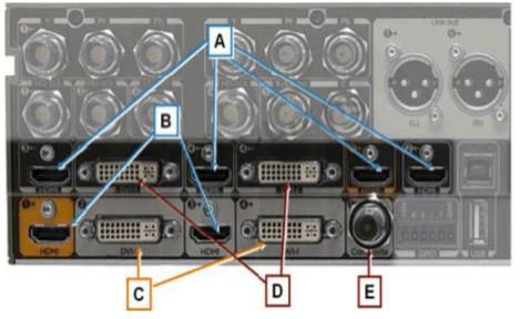
You are installing a high-definition (720p or 1080p) monitor on the Cisco TelePresence Codec C90. Which of the outputs that are represented by letters in the exhibit should you use?
