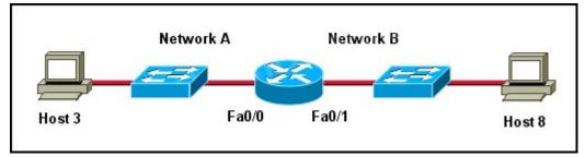
Host 3 on Network A is sending data to Host 8 on Network B.
