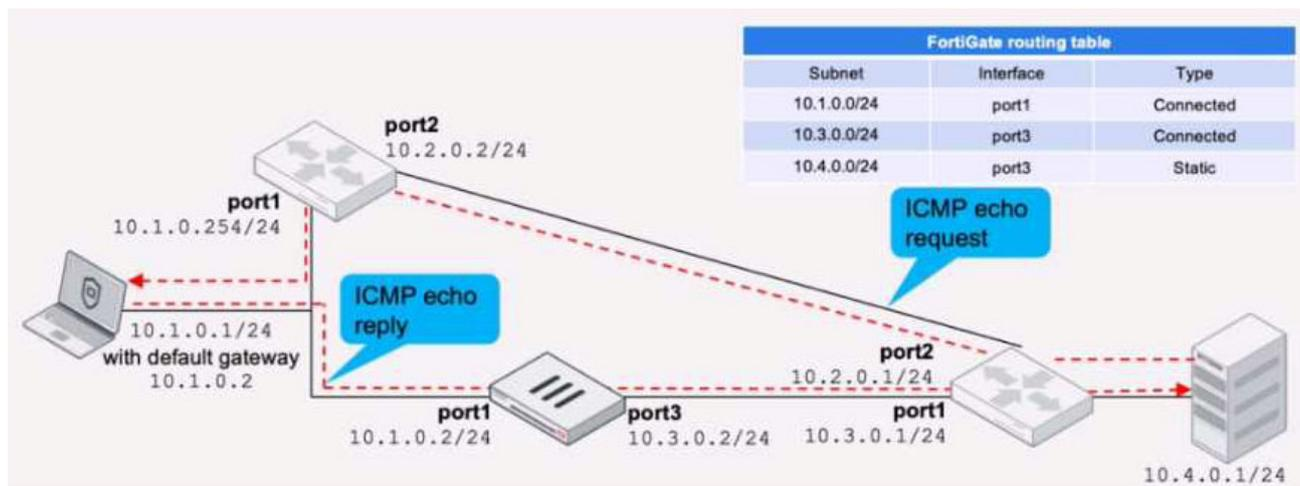
FortiGate has already been configured with a firewall policy that allows all ICMP traffic to flow from port1 to port3.
