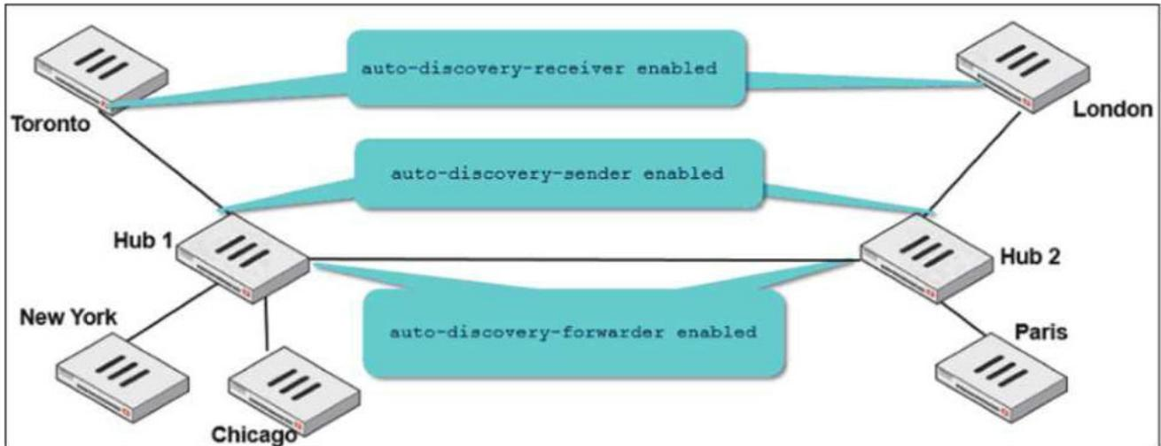
Two hub-and-spoke groups are connected through a site-to-site IPsec VPN between Hub 1 and Hub 2. The administrator configured ADVPN on both hub-and-spoke groups.
