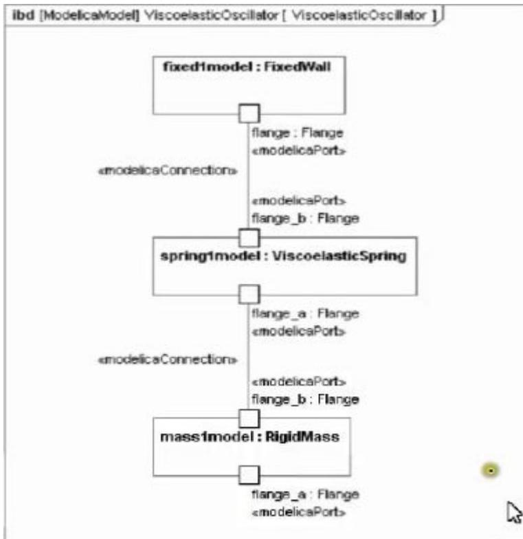
Assume that all stereotypes required by the SysML-Modelica Transformation specification (if any) have been applied but are not necessarily shown here. Assume that FixedWall, ViscoelasticSpring, and RigidMass are fully defined in a Modelica library.
